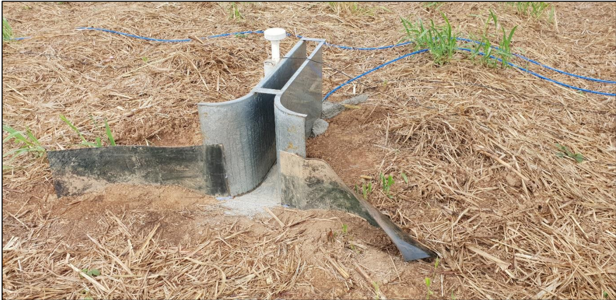
Figure 61. San dumas flume. Rubber bunding is used to direct flow into the flume from between the row mounds. Earth / concrete bunding used to direct water discharge from each adjacent interrow into the interrow with the flume installed approximately 3 metres uphill of the flume. The row profile is approximately 0.2 metres higher than the interrow.
