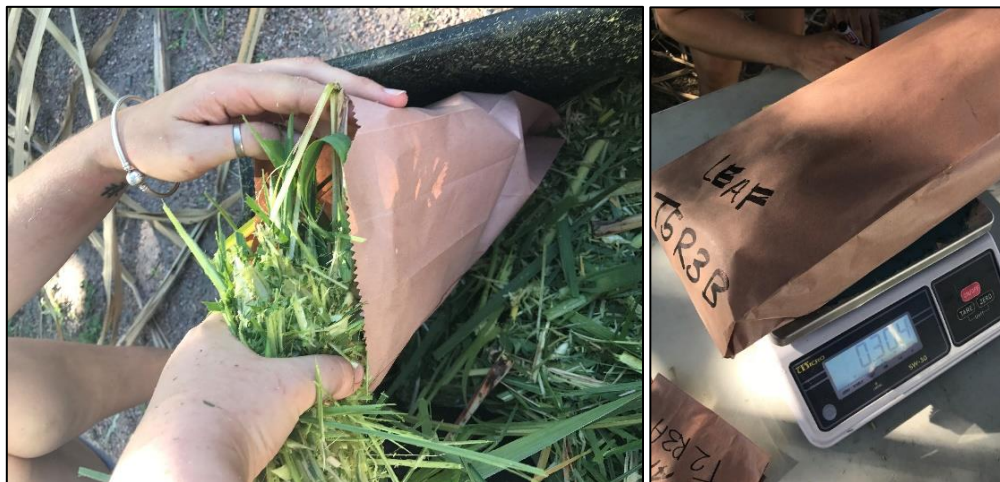
Figure 38. Subsampling and weighing of fresh material
