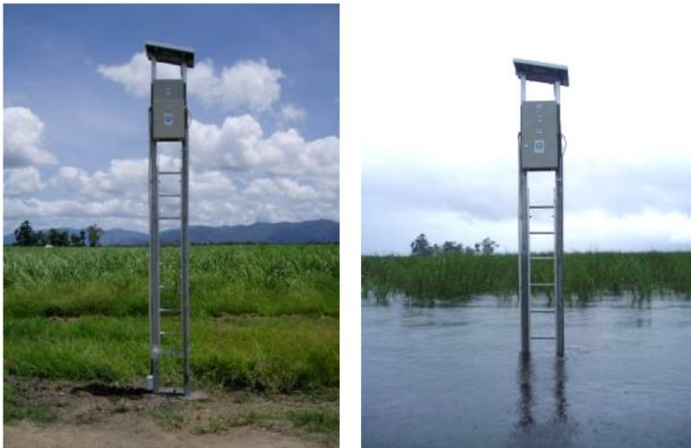
Figure 26: Example of an auto-sampler system installed on the Murray River floodplain (reproduced from Hawdon et al., 2007)
