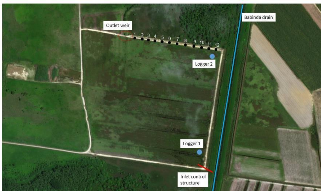
Figure 5: Babinda constructed wetland showing location of the inlet control structure between the wetland and the Babinda drain, position of the diver loggers (Logger 1, Logger 2) recording water depth, water temperature and conductivity, the outlet weir, and the twelve manually control outlet pipes
