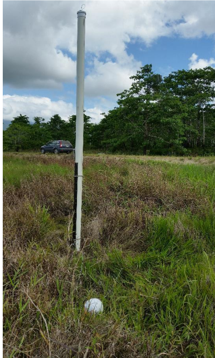
Figure 9: CTV Diver logger configuration in Babinda wetland
