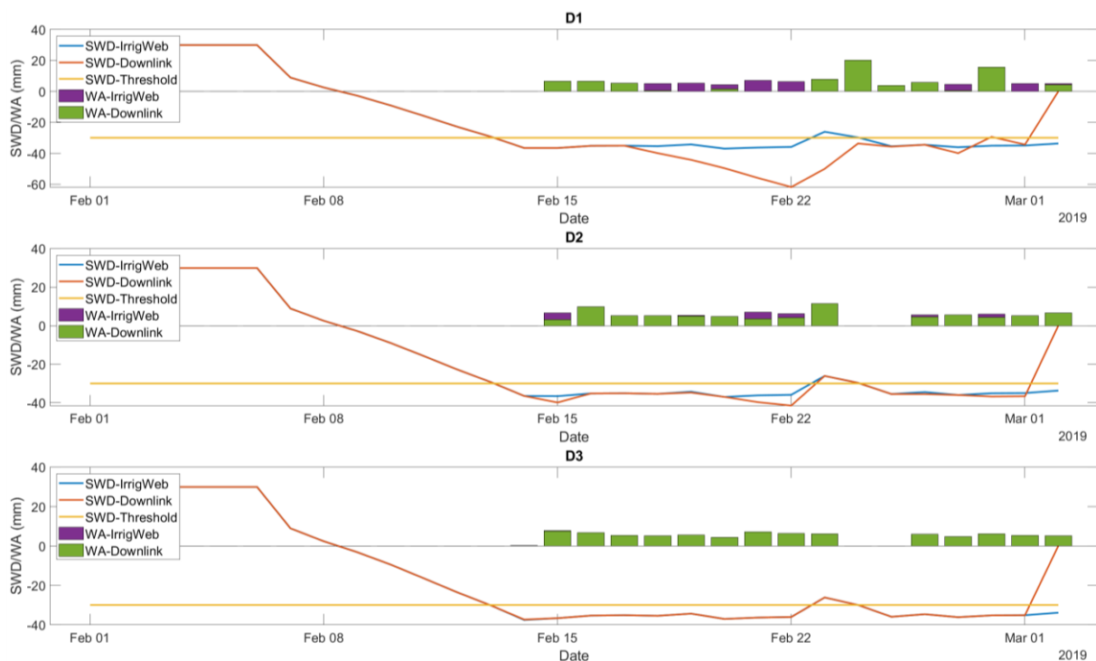
Figure 21: Soil water deficit (SWD) (mm) and water applied (WA) (mm) of drip blocks, i.e. D1, D2 and D3. The orange line represents the SWD threshold that is set up by the farmer to trigger irrigation events. The blue line represents the SWD using IrrigWeb schedules, and the red line is the SWD using Downlink schedules. The green bar represents the WA using Downlink schedules, and the purple bar is the WA if using IrrigWeb schedules.
