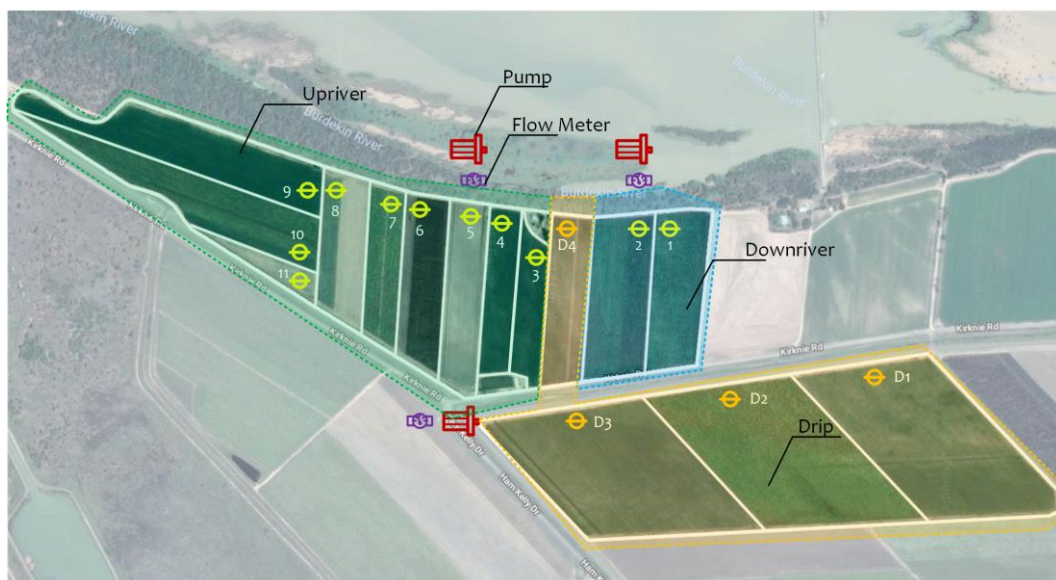
Figure 15: The test farm is divided into three hydraulic groups, i.e., the Upriver and Downriver groups are with furrow irrigation system, and the Drip group is with a drip irrigation system.
