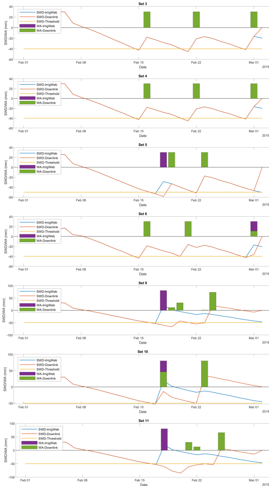
Figure 22: Soil water deficit (SWD) (mm) and water applied (WA) (mm) of furrow blocks, i.e., Set 3, Set 4, Set 5, Set 6, Set 9, Set 10 and Set 11. The orange line represents the SWD threshold that is set up by the farmer to trigger irrigation events. The blue line represents the SWD using IrrigWeb schedules, and the red line is the SWD using Downlink schedules. The green bar represents the WA using Downlink schedules, and the purple bar is the WA if using IrrigWeb schedules.
