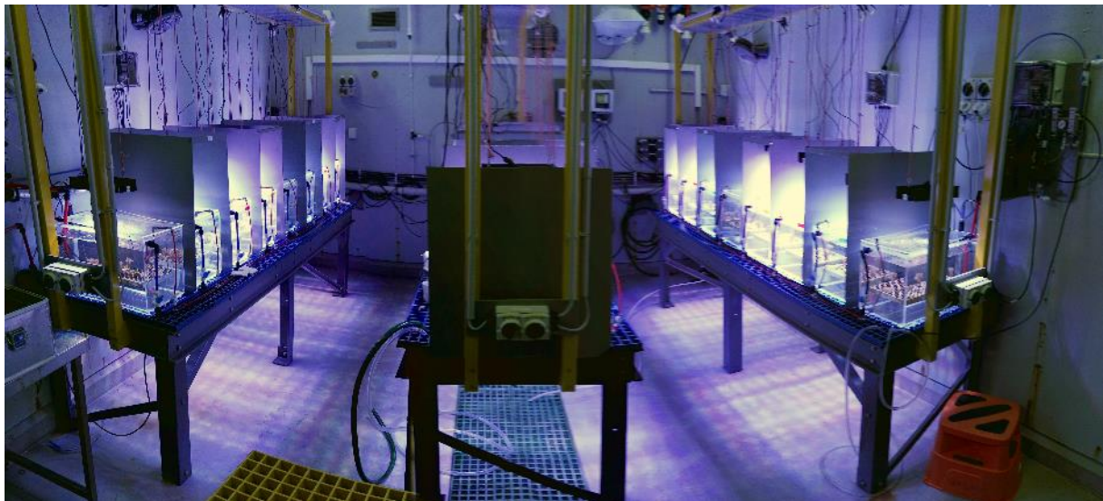
Figure 7: Experimental room to assess the effects of low, variable, medium and high daily light integrals on coral recruits and adults.
