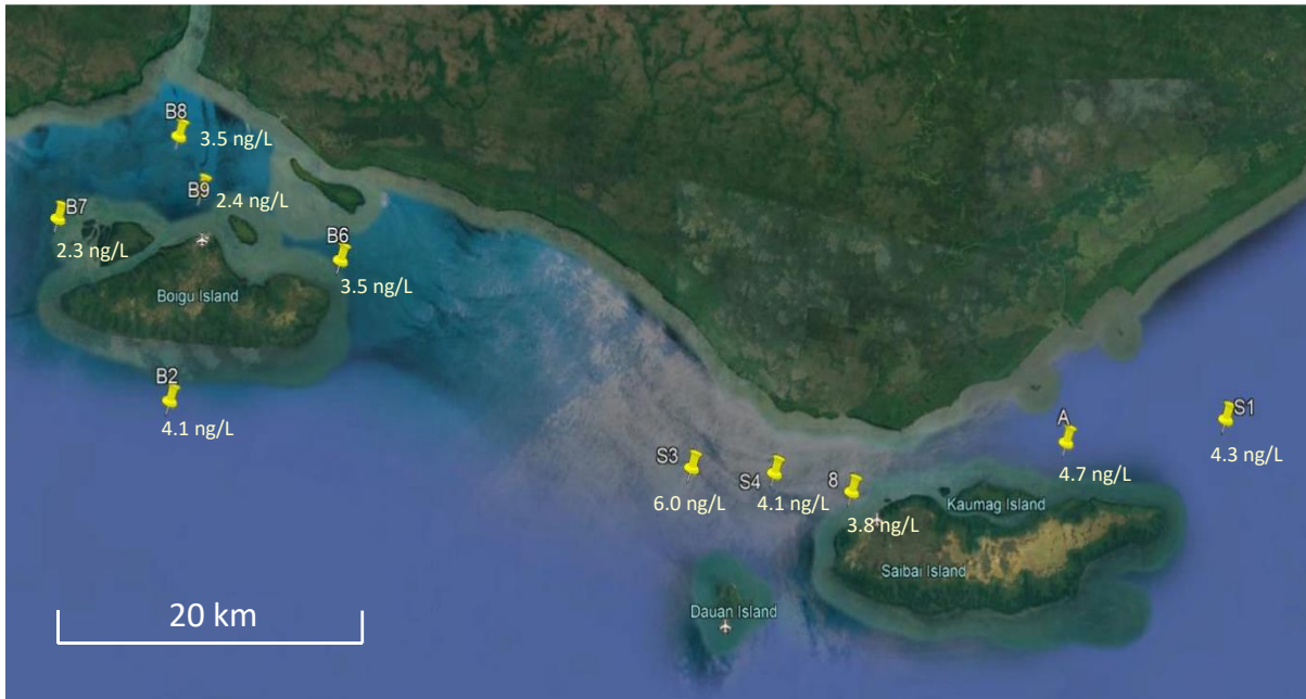
Figure 7–8: Map showing the distributions of dissolved lead concentrations (ng/L) around Boigu and Saibai Islands, December 2019 survey.
