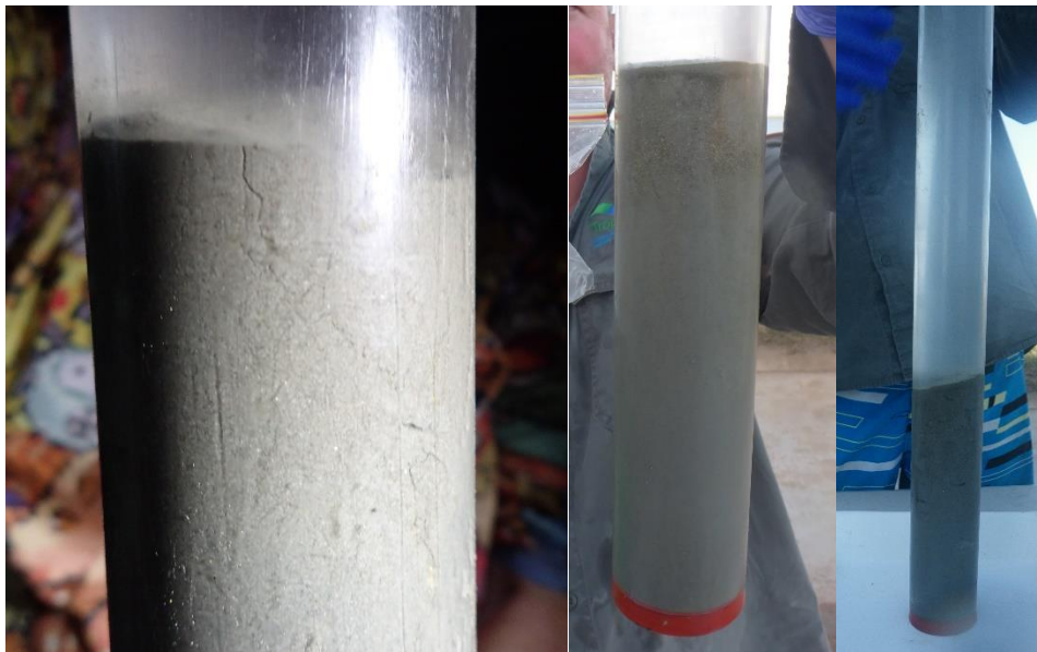
Figure 7–9: Examples of fine sediment cores taken at Boigu (left) and Saibai (middle and right).
