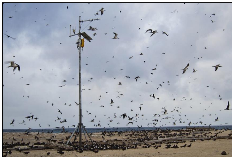
Figure 4–2: Land based component of the Bramble Cay weather station
