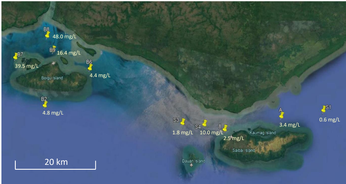
Figure 7-6: Map showing the distributions of suspended sediments (TSS mg/L) around Boigu and Saibai Islands, December 2019 survey.
