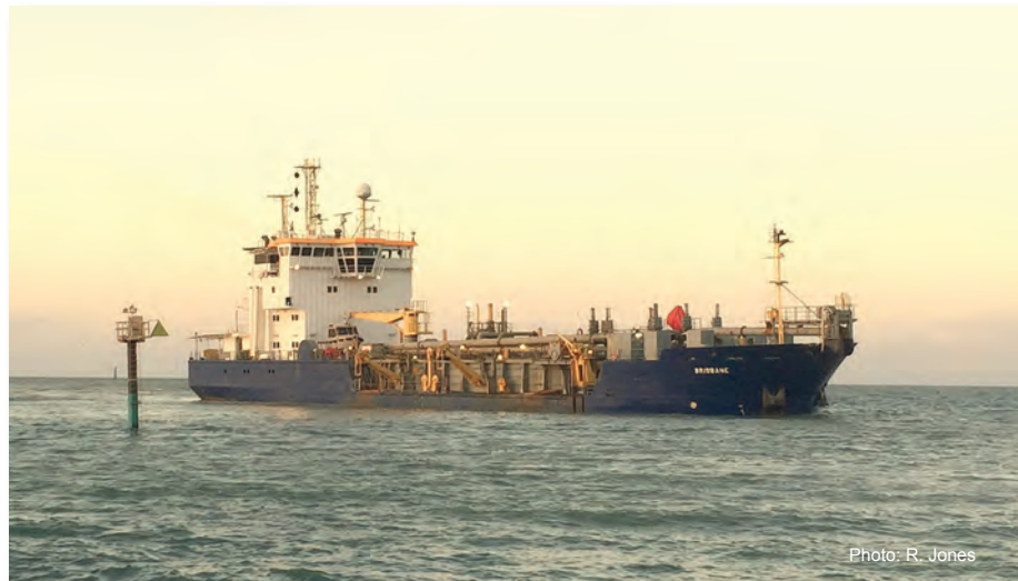
The trailing suction hopper dredge 'Brisbane' in the Port of Townsville in 2015
